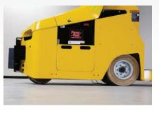
Front Dual Coil Suspension and Rear Coil Suspension with Shock Absorbers
